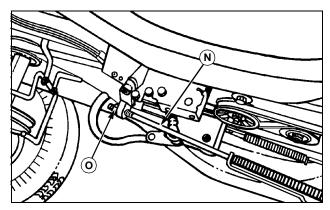
12. Raise tension rod (N) and attach to blade drive arm (O) using flat washer (P) and spring locking pin (Q).
